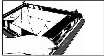
Make sure you correctly slot the frame under the spigot next to the hinge.
