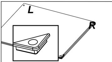
Then replace the door and the 2nd pane, positioning it onto the first.
