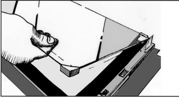
This assembly comprises 2 glass windows, the 1st of which has 2 rubber stops on the 2 front corners.
