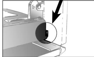
Attach the frame by tightening it with the door. Do not press on the frame alone.
