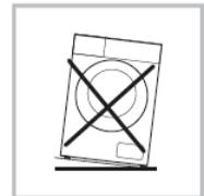
The washing machine is designed to operate at ambient temperature. If it is used in a room where the temperature is below 0°C, the water inlet valve and the drainage system may be damaged.
